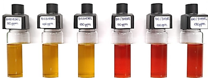
Figure 1. Biodiesel and diesel sample mixed with Al 2 O 3 nanoparticles.
