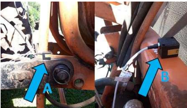
Fig. 2: Accelerometer A located in the hydraulic arm and accelerometer B located in the implement.
