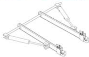
Fig. 1: New quick coupling system between the tractor and the implement.
