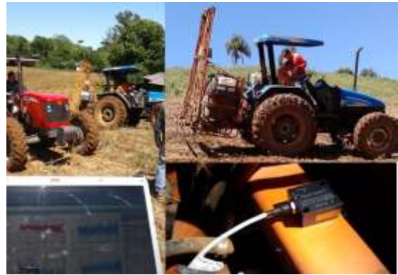
Fig. 3: Test performed for measuring the acceleration in a three-point system.
