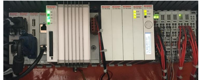
Fig. 7 – PC CX1020 - Beckhoff in operation
